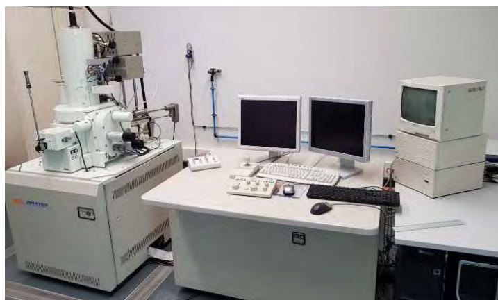
Figure 31 : MEB-FEG JEOL JSM6700F de la plateforme Raimond Castaing, Toulouse
