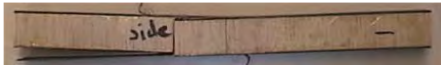
FIGURE 50 – Rupture de composite à âme balsa [Abo00].
