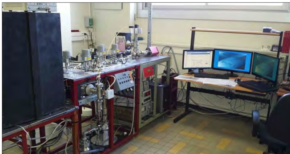
Figure 3.15 – Picture of the Helium line ( http://www.gm.univ-montp2.fr ) in the Laboratoire Geosciences Montpellier. The black box is where is placed the laser, and at the end of the line the quadrupole mass spectrometer.
