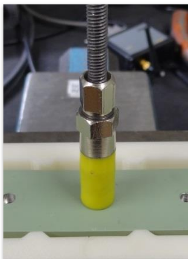
Figure 3.5-5 Fixation temporaire sans ressort
