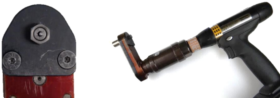
Figure 4.1-1 Visseuse sans fil Atlas Copco ETP-STB32-12-10
