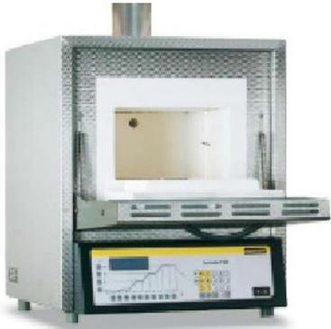
A photograph of a laboratory electric furnace. It is a rectangular metal cabinet with a glass door that is open, revealing a white interior chamber. Below the door is a control panel with a digital display and several buttons. The furnace is standing on four small legs. | <p data-bbox="837 719 1286 882">Four d'incinération<br/>Température maximale à 1100°C<br/>Capacité de 3 litres<br/>Aération évalué à 6 fois par minute</p> |
