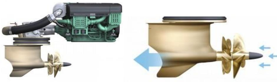
Figure 21: Transmission en pod-drive.
