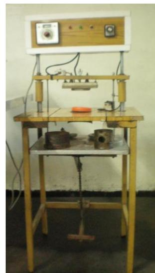
**Figure 14 : Appareil de thermoscellage**
