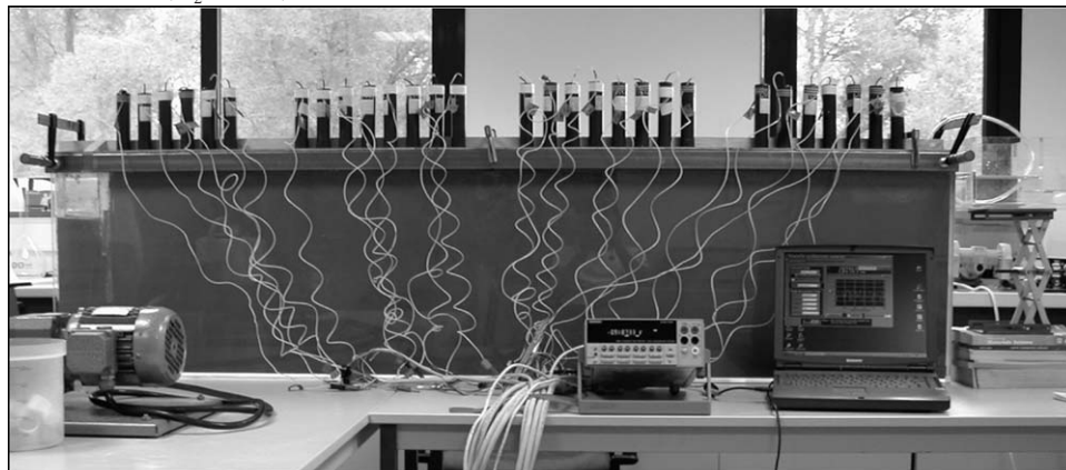
Fig. 2. Picture of the Plexiglas tank. All the electrodes are connected to a multichannel multimeter interfaced to a laptop computer. One electrode is used as a reference (here located on the right side of the picture) for the measurements.
