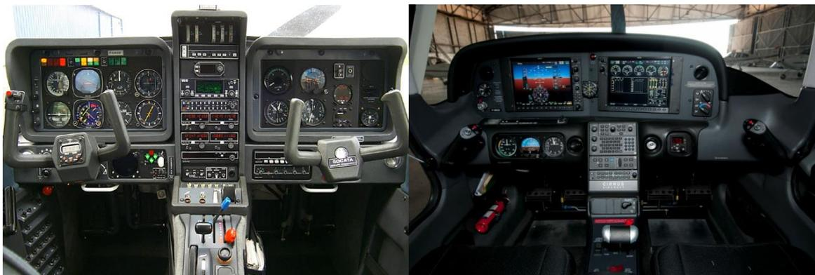
Figure 1 - Cockpit analogique (a) vs *glass cockpit* (b)
