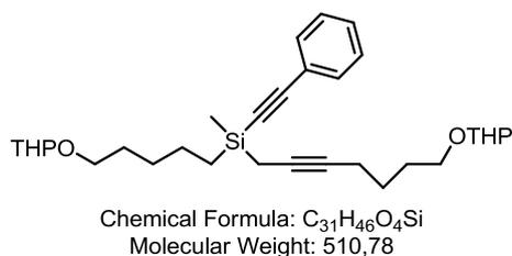
**Methyl(phenylethynyl)(7-(tetrahydro-2H-pyran-2-yloxy)hept-2-ynyl)(5-(tetrahydro-2H-pyran-2-yloxy)pentyl)silane (4)**. To a solution of ethoxysilane **3** (4.636 g, 10.20 mmol, 1 equiv.) in THF (50 mL) was added a solution of lithium phenylacetylide (30.59 mmol, 3
