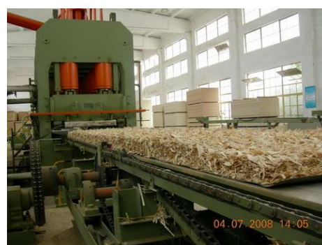
Figure 12: Mechanical Process for Bamboo Fiber Manufacturing. Source: ( www.marginup.com )
