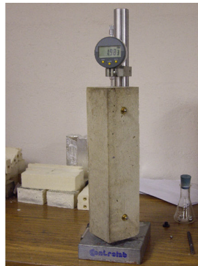
FIGURE B.1: Essais de dessiccation
