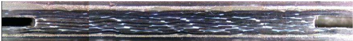
Figure X.12 – Echantillon Arcan-Mines poli miroir avant essai
