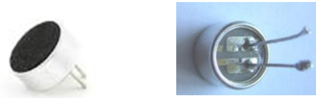
Figure 3.6 : Le microphone Electret
