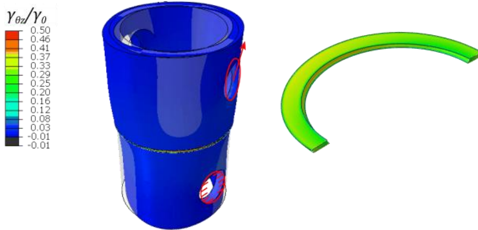
Figure 17: Deformed state of the napkin ring test
