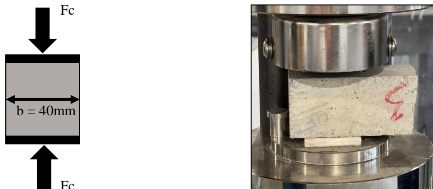
Figure II-24: Essai de compression
