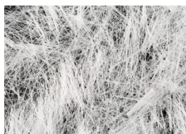
Figure I-20: Les fibres polypropylènes
