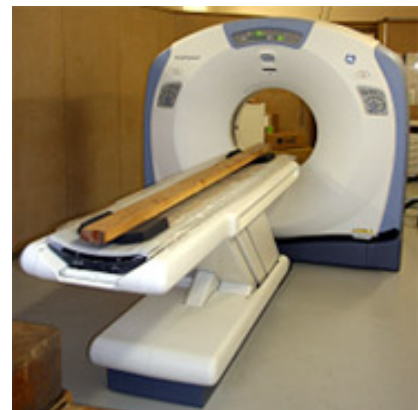
Photo II.21 : Scanner Medical General Electric Brightspeed Exel (INRA).
