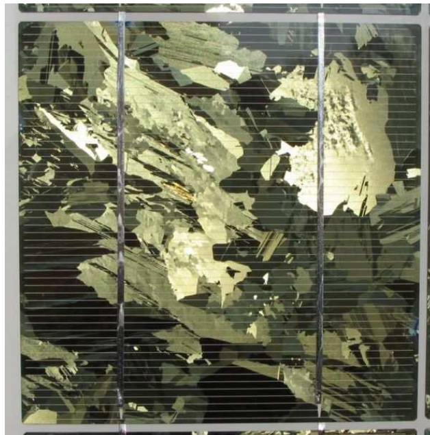
Figure 22 : Structure polycristalline (source : imex.cgi.fr)
