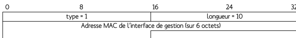
FIG. 3.6: Le TLV "Device-id"
