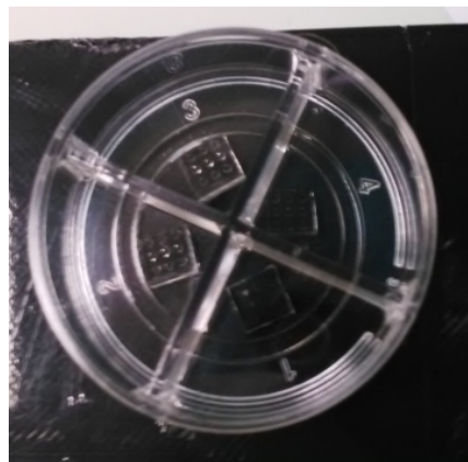
4 arrays of 9 microdevices glued in a 35mm culture plate
