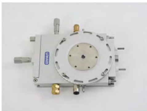
FIGURE 2.29 – Platine chauffante Linkam THMS 600
