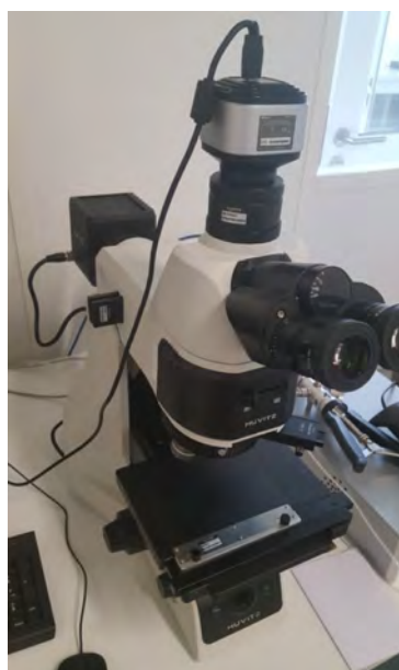
FIGURE 2.30 – microscope optique Huvitz HRM 300
