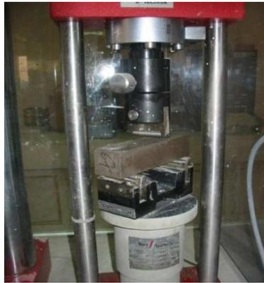
FIGURE 23: MACHINE D'ESSAI DE RESISTANCE À LA FLEXION [Doc]
