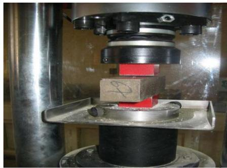
FIGURE 24: MACHINE D'ESSAI DE RESISTANCE À LA COMPRESSION [Doc]
