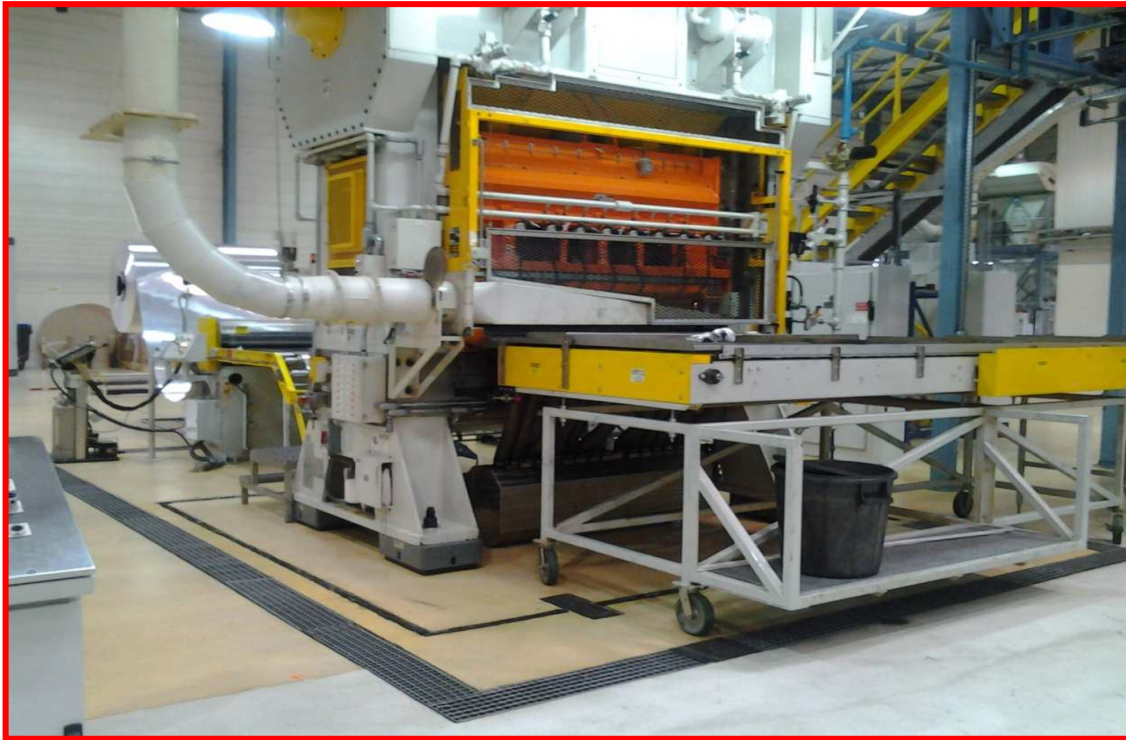
Figure 3 : Presse verticale (Cupper)
