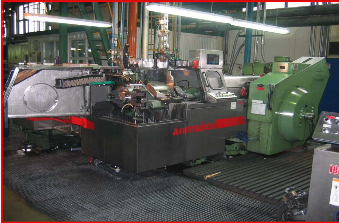
Figure 4 : Presse Horizontale (Bobymaker)
