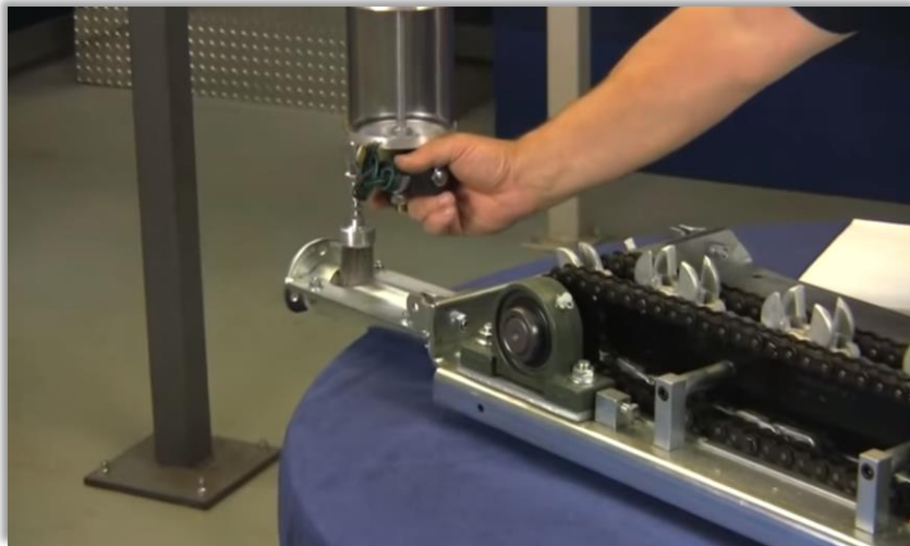
Figure 48: Emplacement lubrification Caterpillar drive
