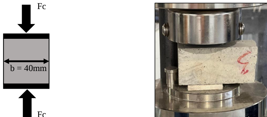
Figure II-24: Essai de compression
