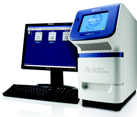
Figure 3 : Thermocycleur Applied Biosystem-StepOne.
