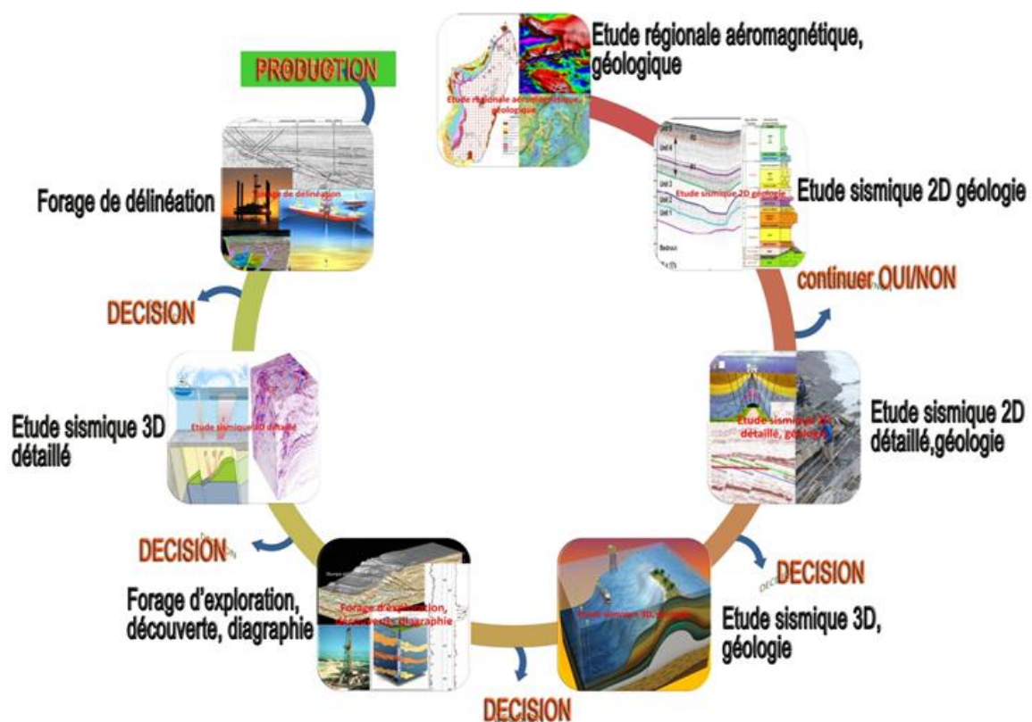
Figure 6: Etapes de prospection pétrolière (Source : OMNIS)
