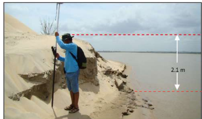
Figure 3. The banks of the mid-channel bar (study area) are associated with highly erodible unconsolidated deposits.
