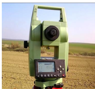
Photo 5: La station total Leica TCR303
