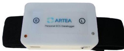
Figure 1.9 : Data logger (ECG) [30].
