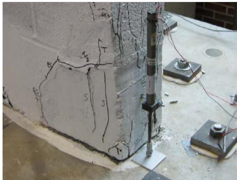
**Figure 4-9 – Mounting of an edge uplift potentiometer (Source: Wight 2006)**
