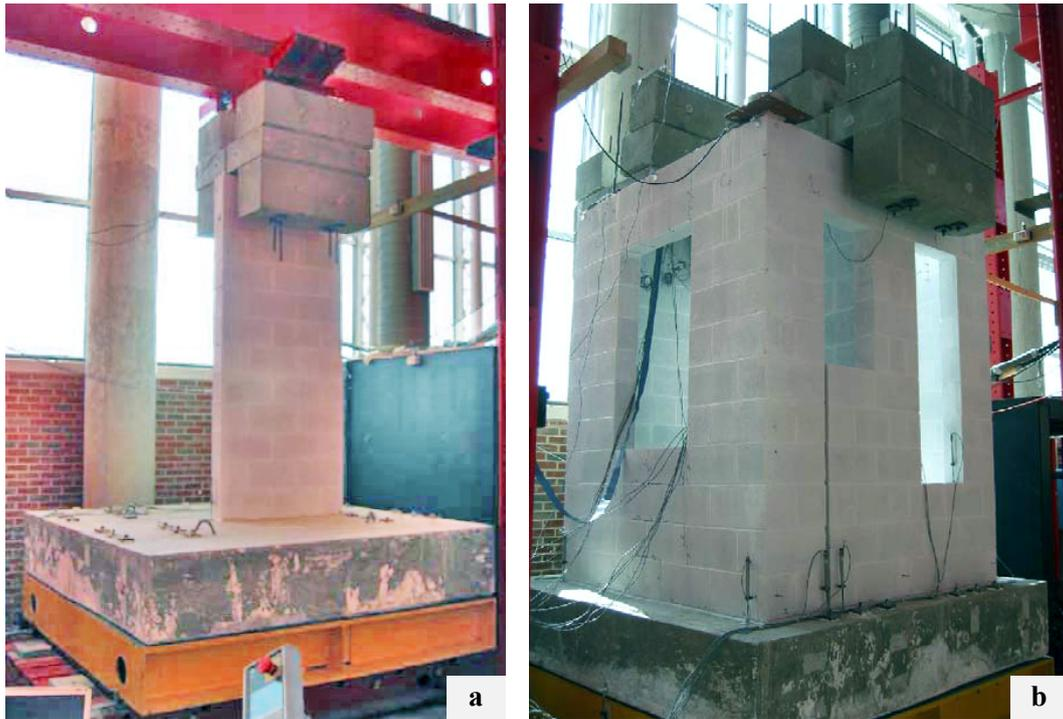
Figure 4-3 – a) Typical single PCM wall specimen and b) PCM structure on the shake table (Source: Wight 2006)
