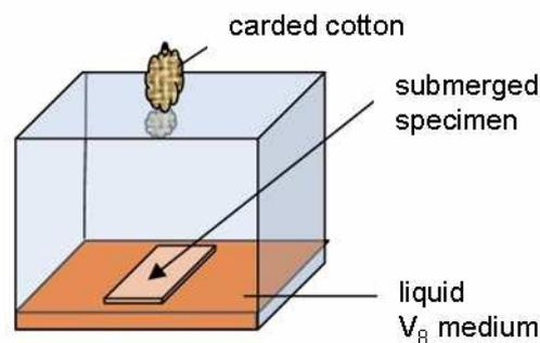
Figure 45: Experimental device developed for the 1<sup>st</sup> test
