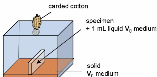
Figure 46: Experimental device for test B
