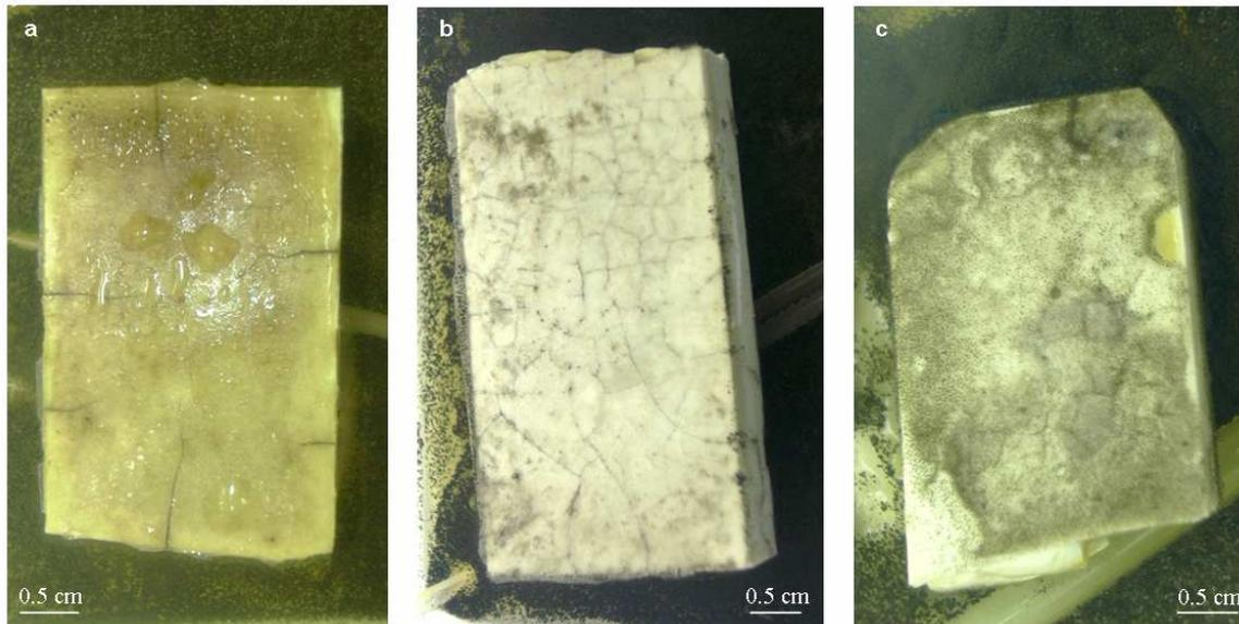
**Figure 51: Observations of specimens inoculated with *Aspergillus niger* after 10 days of incubation at  $24\pm 1^\circ\text{C}$  and  $75\pm 5\%$  RH – (a) Non weathered specimen, (b) carbonated specimen, (c) carbonated then leached specimen**
