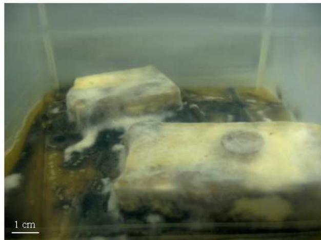
**Figure 52: Observations of carbonated and leached specimens inoculated with *Alternaria alternata* after 10 days of incubation at  $24\pm 1^\circ\text{C}$  and  $90\pm 5\%$  RH**
