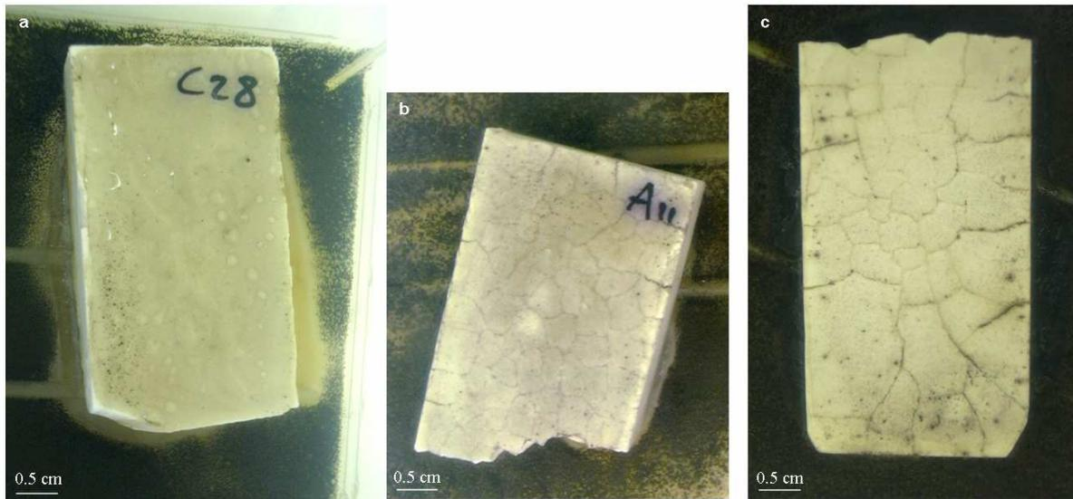
**Figure 49: Observations of specimens inoculated with *Aspergillus niger* after 10 days of incubation at  $24\pm 1^\circ\text{C}$  and  $75\pm 5\%$  RH – (a) Non weathered specimen, (b) carbonated specimen, (c) carbonated then leached specimen**
