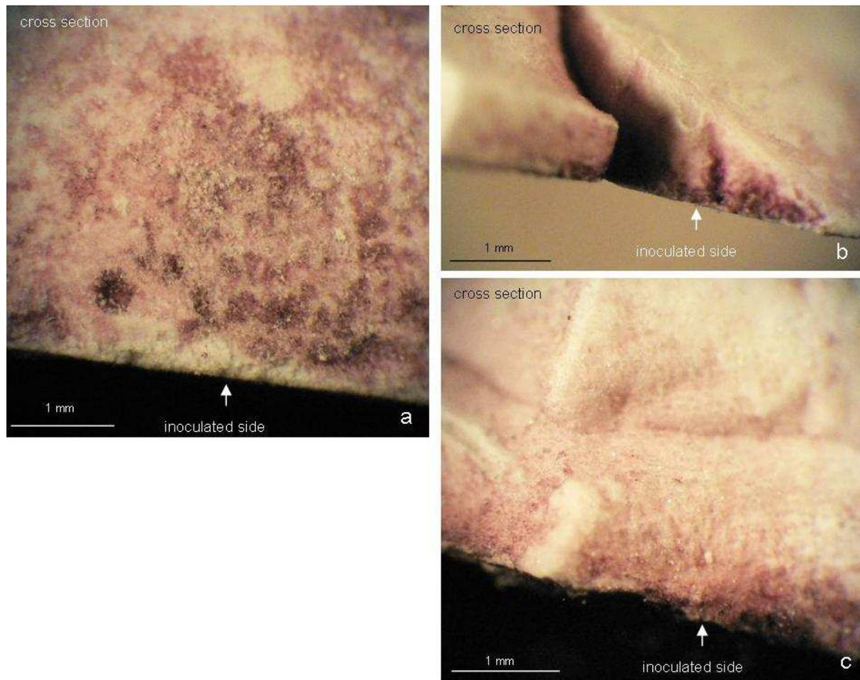
**Figure 64: Observations with stereomicroscope of cross-sections details of carbonated then leached specimen after the PAS staining – (a) inoculated with *Aspergillus niger*, (b) control, (c) inoculated with *Coniosporium uncinatum***
