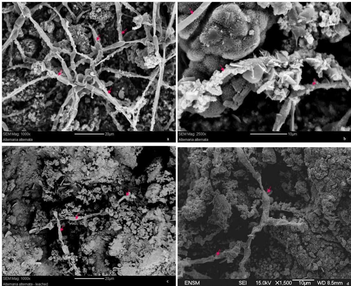
**Figure 68: SEM observations of specimens inoculated with *Alternaria alternata* – (a), (b) surface observation of the carbonated specimen; (c) observation of the cross section of the carbonated then leached specimen, (d) observation of the cross-section of the carbonated specimen**
