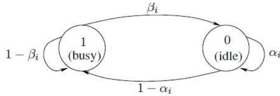
FIGURE 4.3: The channel transition probabilities for channel  $i$ .
