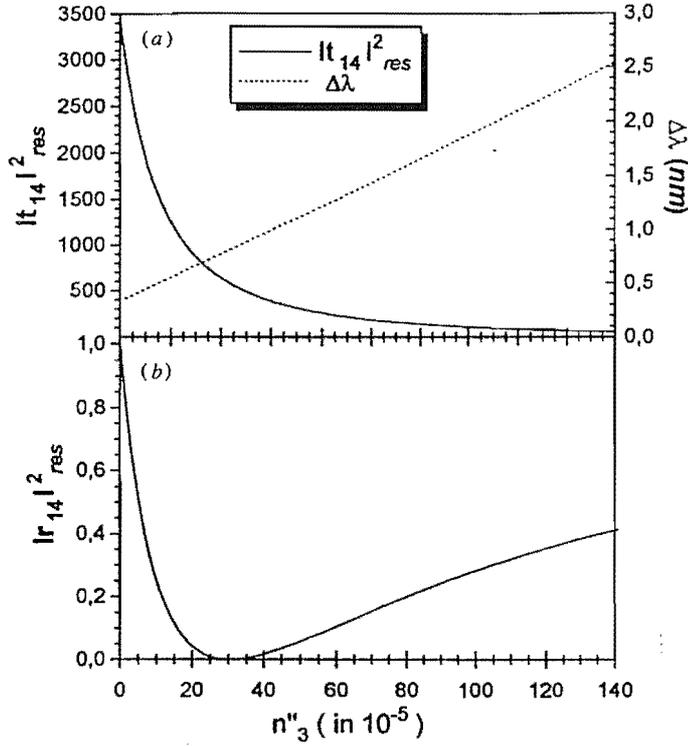
Figure 6. On-resonance transmission  $|t_{14}|_{res}^2$  and (a) resonance width  $\Delta\lambda$  and (b) on-resonance reflection  $|r_{14}|_{res}^2$  as a function of  $n''_3$ . These curves are plotted using the results of the Lorentzian approximation, with the nominal values of the parameters of the structure (see figure 1).
