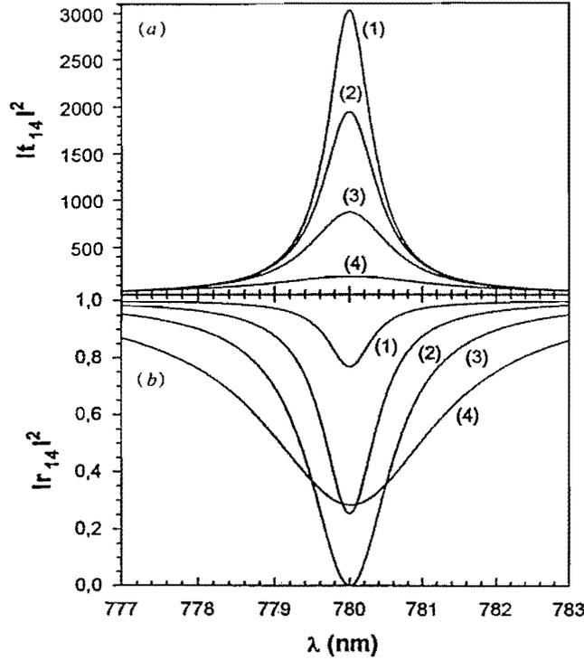
Figure 3. (a) transmission factor  $|t_{14}|^2$  and (b) reflection coefficient  $|r_{14}|^2$  as a function of the wavelength in the presence of losses. The gap thickness is fixed ( $d_2 = 700$  nm) and the losses, included through an imaginary part of the index of refraction of the waveguide, are varied. (1)  $n_3'' = 2 \times 10^{-5}$ ; (2)  $n_3'' = 10^{-4}$ ; (3)  $n_3'' = 3 \times 10^{-4}$ ; (4)  $n_3'' = 10^{-3}$ .
