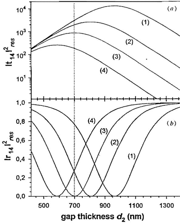
Figure 4. (a) On-resonance transmission factor  $|t_{14}|_{res}^2$  and (b) reflection coefficient  $|r_{14}|_{res}^2$  as a function of the gap thickness  $d_2$ , for different values of the losses. The values of  $n_3''$  are the same as in figure 3. (1)  $n_3'' = 2 \times 10^{-5}$ ; (2)  $n_3'' = 10^{-4}$ ; (3)  $n_3'' = 3 \times 10^{-4}$ ; (4)  $n_3'' = 10^{-3}$ . The dotted vertical line at  $d_2 = 700$  nm corresponds to the conditions of figure 3.
