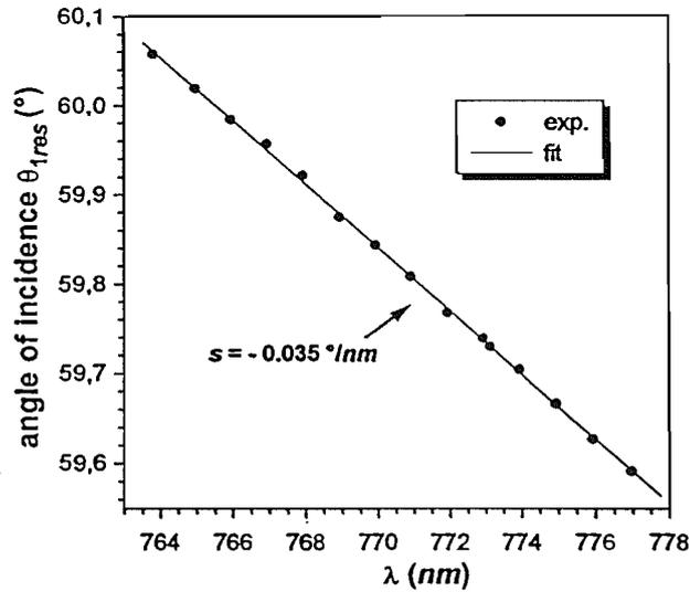
Figure 9. Measurement of the variation of the resonance angular position  $\theta_{1\text{res}}$  with the wavelength  $\lambda$ . The slope  $s$  of this curve is used for the deconvolution of the experimental data. Our set-up did not permit the measurement of the angle of incidence around  $\lambda_{\text{res}} = 780$  nm. The linearity of the curve over the 15 nm range shown allows us to extrapolate to the value at  $\lambda_{\text{res}} = 780$  nm.
