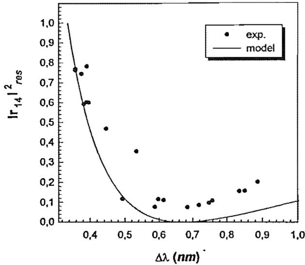
**Figure 11.** Measured values of  $|r_{14}|_{res}^2$  versus  $\Delta\lambda$  at various points during nine months of the prism's history. The measured on-resonance reflection coefficient  $|r_{14}|_{res}^2$  is plotted as a function of the measured width of the resonance  $\Delta\lambda$  (filled symbols). The full curve corresponds to the theoretical evolution when only  $n_3''$  is varied.
