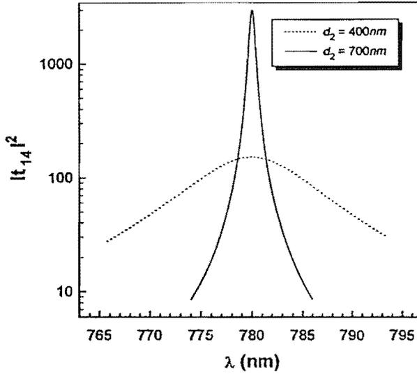
**Figure 2.** Resonant behaviour of the transmission factor  $|t_{14}|^2$  in the loss-free case, as a function of the wavelength, for two values of the gap thickness  $d_2$ .  $t_{14}$  is the ratio of the electric field amplitudes in the evanescent wave and in the prism, as defined in equation (11). The resonance is more pronounced when the gap is thicker.
