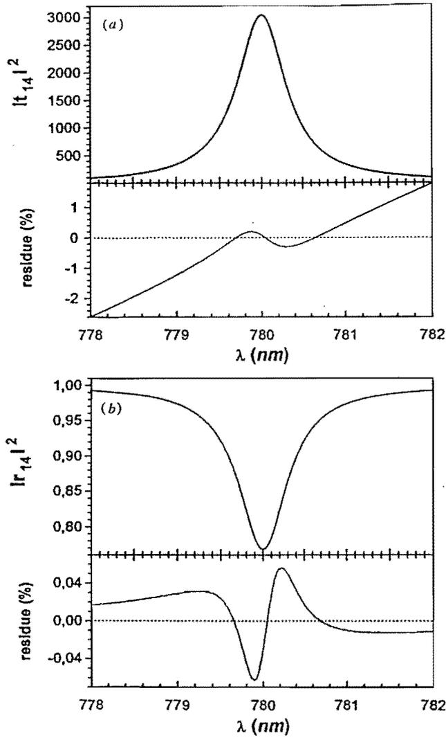
Figure 5. Comparison between the results of the exact calculation (equations (13) and (16)) and the Lorentzian approximation, (a) for the transmission factor  $|t_{14}|^2(\lambda)$  and (b) the reflection coefficient  $|r_{14}|^2(\lambda)$ . For these curves,  $d_2 = 700$  nm and  $n_3'' = 2 \times 10^{-5}$ . The curves are not distinguishable on this scale; the relative differences (residues) are plotted below each curve.
