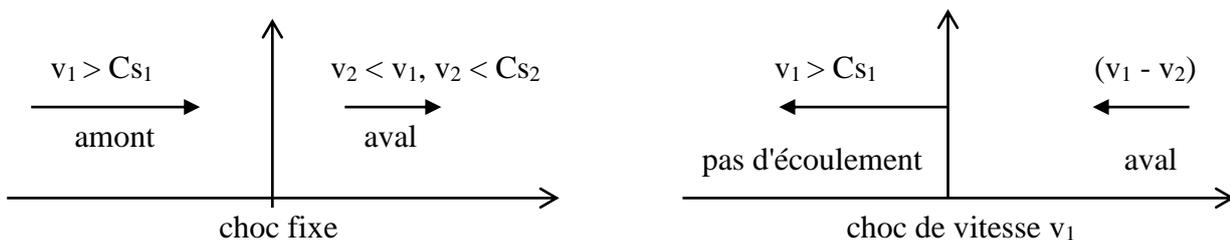
$$v_1/v_2 = \rho_2/\rho_1 = (\gamma+1) M_1^2 / [2 + M_1^2 (\gamma-1)] > 1$$
