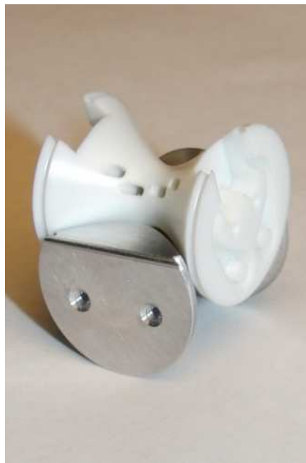
Figure 5.2: Hyperboloid joint of the finger base
