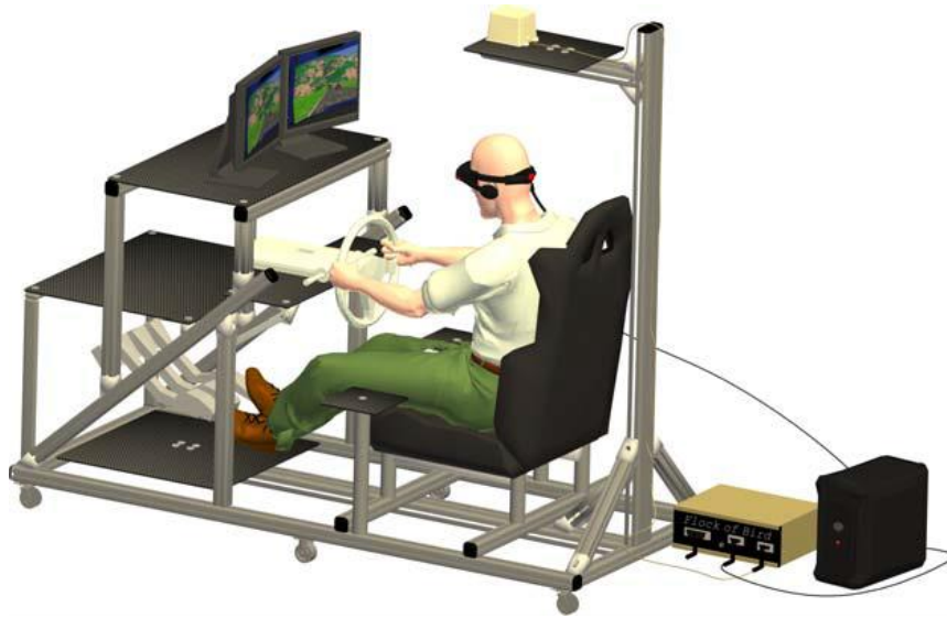
Figure 21: Overview of the set-up. Participants sat on a play seat integrated into an aluminum frame and wore a head mounted display. They controlled the velocity of the virtual car with accelerator and brake pedals and lateral excursions between lanes with the steering wheel. Participants' head pitch, yaw and roll orientations were measured with an electromagnetic tracker and coupled to the visual scene. Participants could also display rear mirrors by pressing buttons on the steering wheel.
