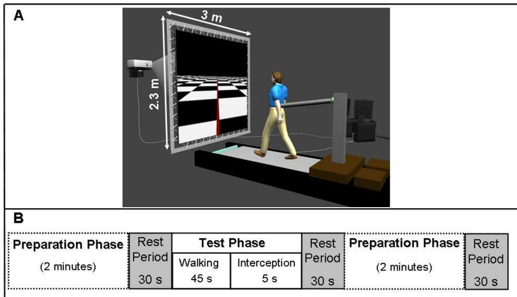
**Figure 41 :** (A) Overview of the virtual reality set-up and the visual scene that was projected onto the screen in front of the participants; (B) Representation of the different phases of the experiment.
