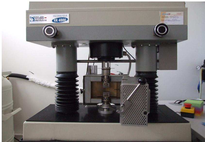
FIGURE 1.20 – DMA Metravib 4400
