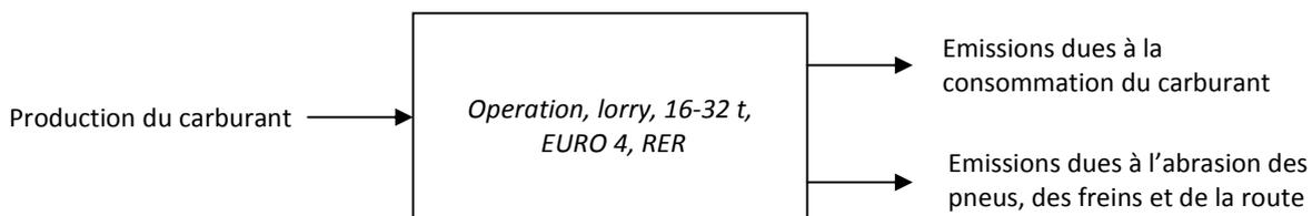
Figure 25 : Description du module "*Operation, lorry 16-32t, EURO 4, RER*"
