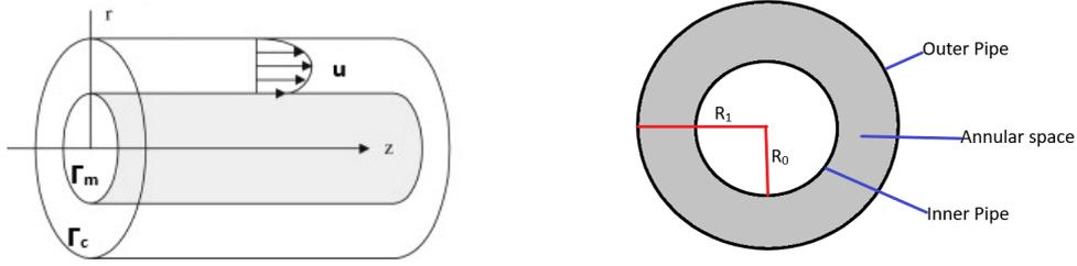
Figure 3.1: Schematic description of annular space bounded by concentric pipes (radius of the inner pipe:  $R_0$  and radius of the outer pipe:  $R_1$ ).
