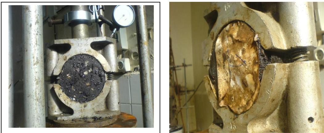
Figure 5.17: Essai de Marshall
