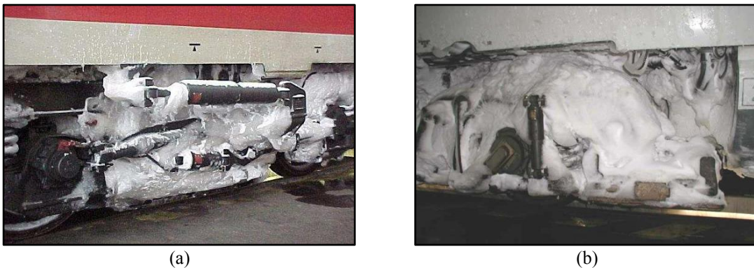
Figure 5. (a-b) Wet-snow accretions on bogies train [18].
