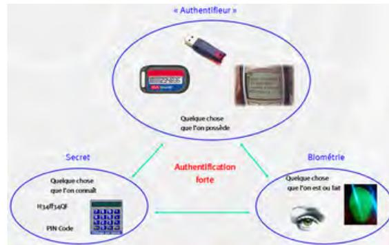
Figure 8.1 – Principe d'authentification forte
