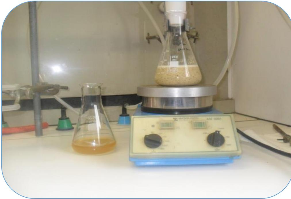
**Photo 10** : *Montage extraction solide/liquide*
