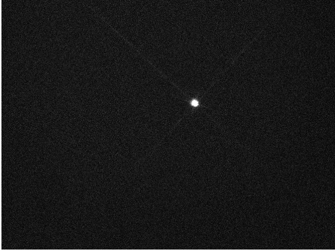
Fig. 3 Image of Deneb , with the Generation 1.5.1 testbed in the 740 – 900 nm bandpass. The central lobe and the diffraction spikes of the primary array are clearly visible. A secondary set of spikes is also visible, originating from diffraction by the spider of the zero order mask.
