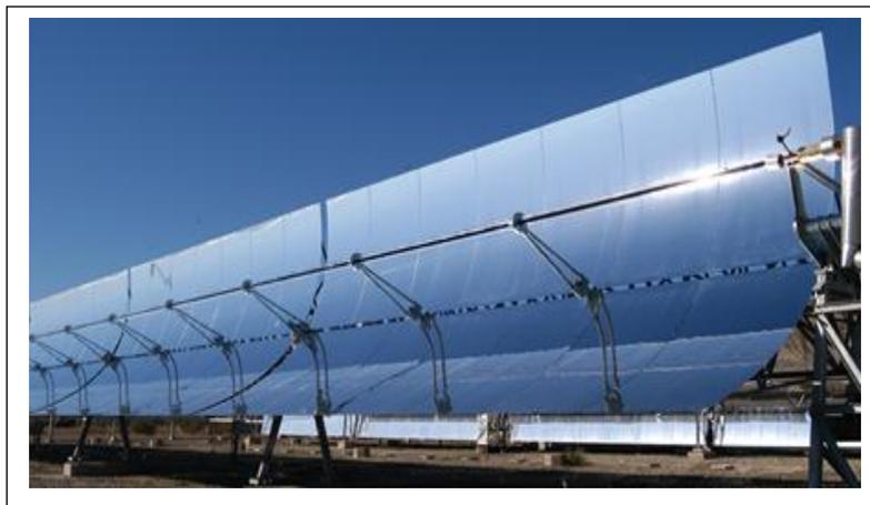
*Fig1.13 Miroir cylindro-parabolique*
