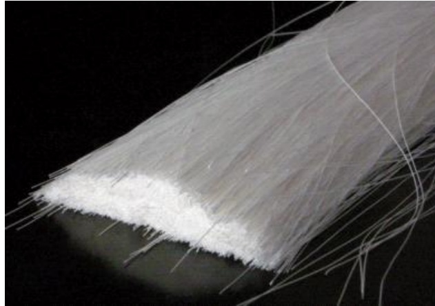
Figure I.10: Membrane en poly sulfone [11]
