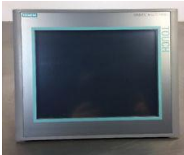
Figure 40 : Panel de supervision.
