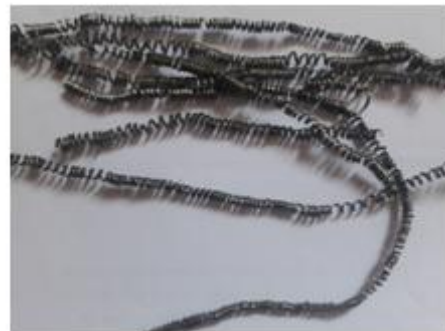
(m) : V_c = 50\text{m/min} p = 1.5\text{mm} a = 0.64\text{mm/tr}
