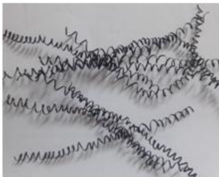
(n) : V_c = 110\text{m/min} p = 2\text{mm} a = 0.4\text{mm/tr}
