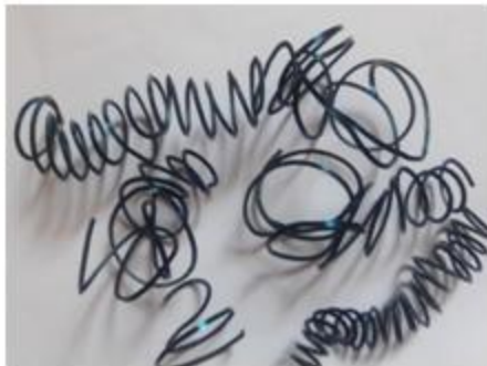
(l) : V_c = 90\text{m/min} p = 0.5\text{mm} a = 0.4\text{mm/tr}
