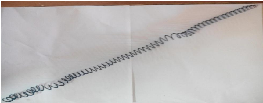
(c) : V_C = 50 m/min P = 2 mm a = 0.8 mm/tr
