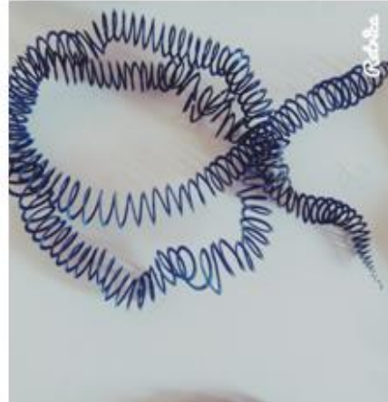
(b) : V_C = 90 m/min p = 0.11 mm a = 1.5 mm/tr
