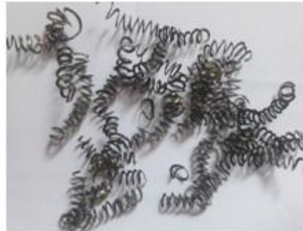
(o) : V_c = 130\text{m/min} p = 2\text{mm} a = 0.64\text{mm/tr}
